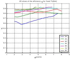
Figure 16: Evolution of the efficiency of the Yamaha PAS as a function of rotational speed for different cyclist's torques
