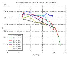
Fig. 22: The assistance factor of the Sachs in 3<sup>rd</sup> speed as function of speed for different cyclist's forces.
