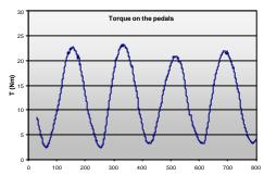
Figure 6: Torque on the pedals during cycling
