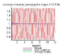
Figure 7: Evolution of the error by averaging the torque signal for f=0.31Hz and f=2.5Hz
