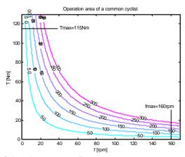
Figure 4: operation area of the (dummy) cyclist
