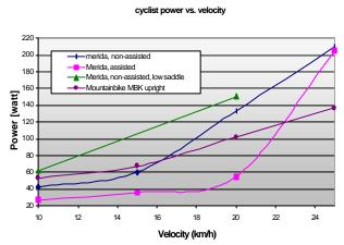
Figure 3: power output vs. velocity for 4 different road tests.
