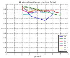
Fig. 21: Evolution of the efficiency of the Sachs as a function of rotational speed for different cyclist's torques.
