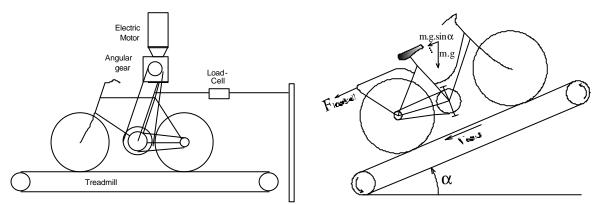
Figure 5: Construction of the test bench
